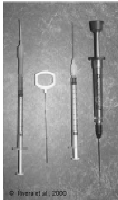
Figure 12. Some instruments used to pick up embryos and oocytes. From left to right are 1) a 1 cc syringe with an extension of rubber tubing connected to a Unopette , 2) a wiretrol (from Drummond Scientific; we purchase from Fisher ), 3) the same device as #1 without the rubber tubing extension and 4) a 5 ml Drummond Microdispenser (also purchased from Fisher ). For tips on how to use these instruments, click here .
